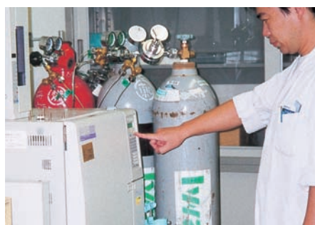
ガスクロマトグラフによる生理活性成分の分析 Analysis of physiologically active components with the use of gas chromatography
